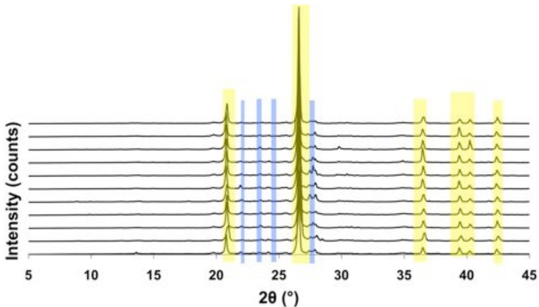
**Figure 4.** X-ray powder diffraction patterns of bulk soil (including sand, silt, and clay particle size fractions) from all sampling areas. Peak positions of dominant minerals shown by color: blue represents feldspar and yellow represents quartz.
