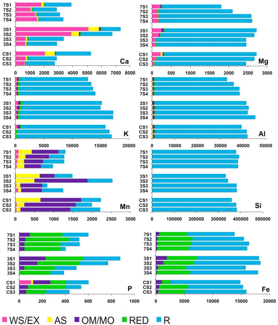
**Figure 5.** Major element release during sequential extractions. Concentrations (in ppm) shown on x-axis. (WS/EX: Water soluble/exchangeable fraction; AS: Acid Soluble fraction; OM: Organic Matter fraction; RED: Reducible fraction; R: Residual fraction). Plots arranged according to trends in distribution among elemental reservoirs.
