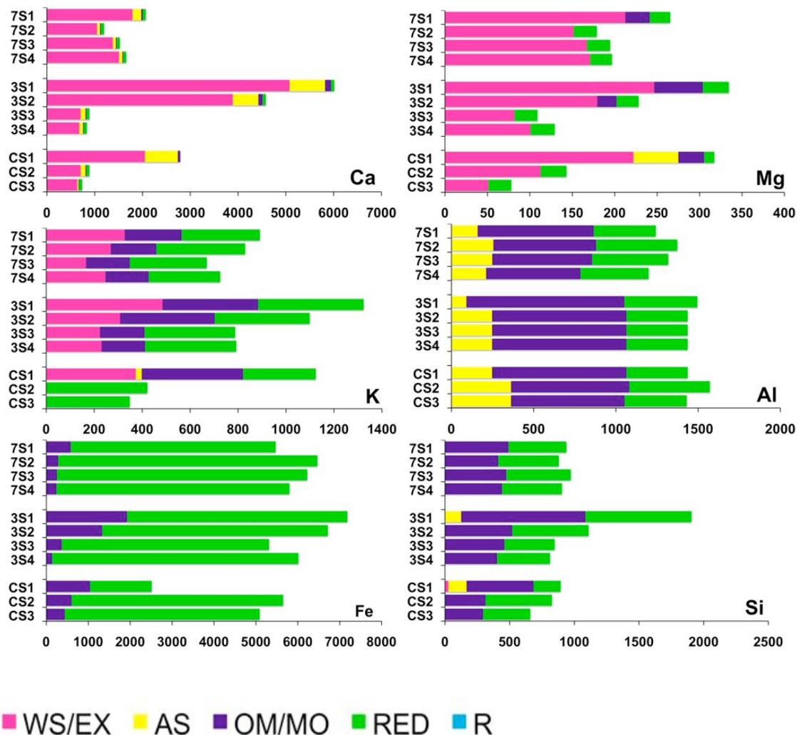
**Figure 6.** Major element release during sequential extractions shown without residual fraction (R). Concentrations (in ppm) shown on x-axis. (WS/EX: Water soluble/exchangeable fraction; AS: Acid Soluble fraction; OM: Organic Matter fraction; RED: Reducible fraction; R: Residual fraction. Plots arranged according to trends in distribution among elemental reservoirs.
